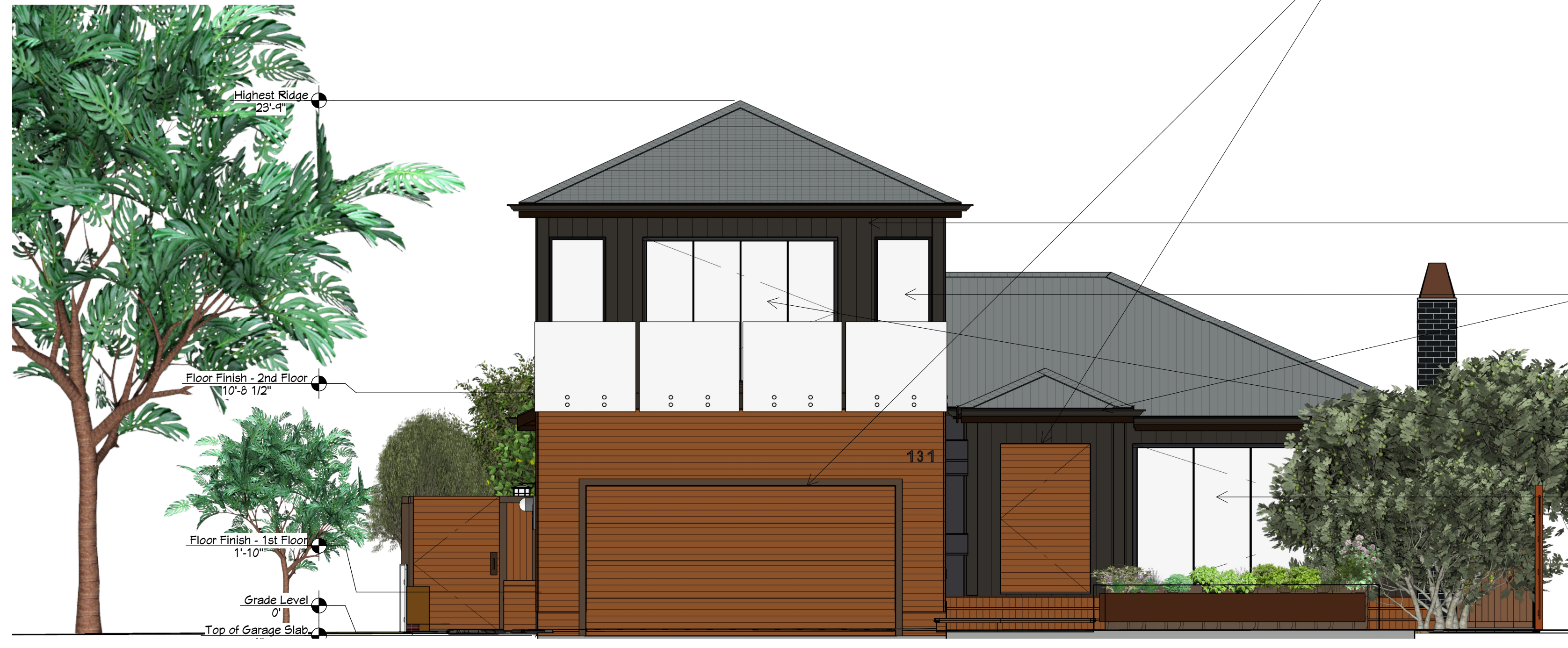
1. New South Elevation 1/4 in = 1 ft
