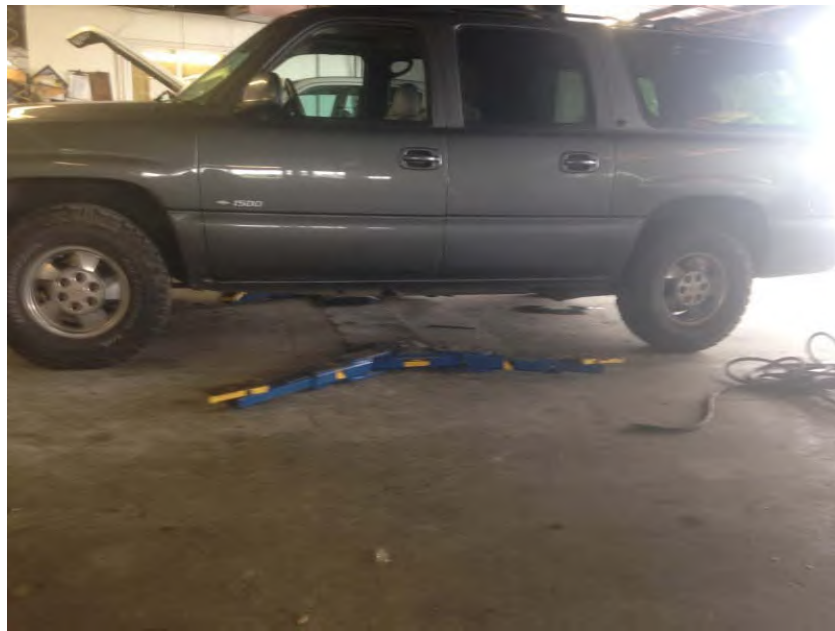
Photo 1. 920 Bayswater Avenue - View of one of two active in-ground hydraulic lifts. Photograph taken April 26, 2017.
