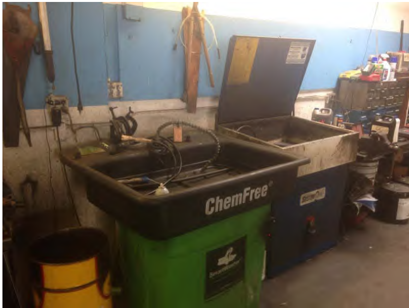
Photo 2. 920 Bayswater Avenue - View of aqueous parts washers. Photograph taken April 26, 2017.
