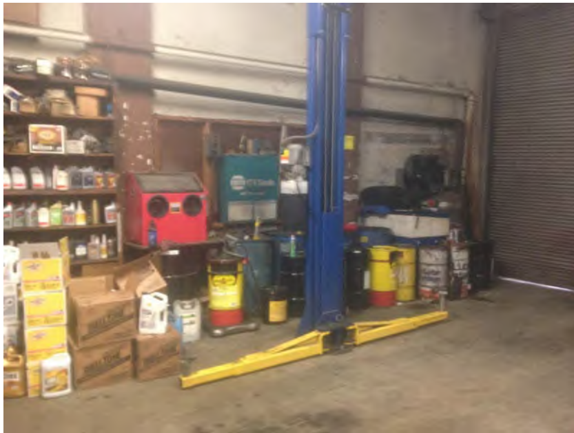
Photo 2. 920 Bayswater Avenue - View of abrasive blasting cabinet, grit storage drum, and small-quantity automotive fluid storage at northeastern property boundary. Photograph taken April 26, 2017.
